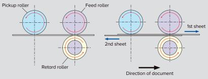
Canon's revolutionary feeding mechanism with retard roller achieves highly reliable page separation.
