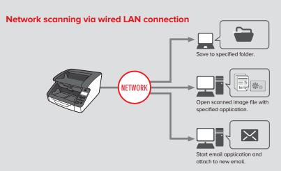
Share a single scanner via a network to perform scanning tasks efficiently. Select any connected computer from the scanner's operation panel and perform scanning. Scanning can also be executed from any computer sharing the scanner via the network. You can save scanned data to specified storage locations, attach scanned data to emails for sending, and perform various scanning operations according to the scan settings configured on each computer.
