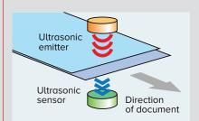
Ultrasonic sensors detect the gap between overlapping pages and prevent multiple pages from being fed together, reliably ensuring that each page of a document is scanned.
