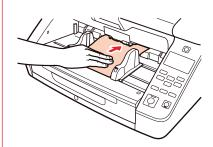
Manual feed mode allows you the option of manually loading sheets of a document for processing.
